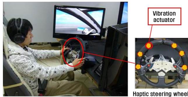
Figure 2 Haptic steering wheel (Yellow circles are locations of vibration actuators)
