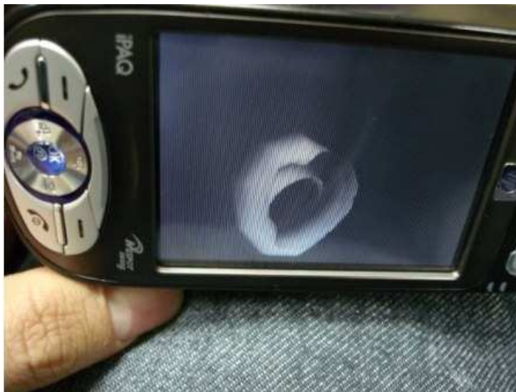
Fig. 3.7 The autostereoscopic display using parallax barrier and stencil buffer algorithm
