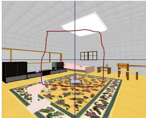
Fig. 4.5 Measuring the perceived FOV. The subjects were asked to mark along the horizontal and vertical lines the extent one felt one was able to see through the display.
