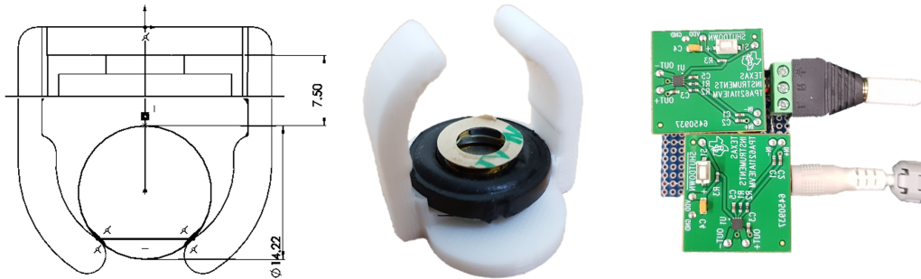
Figure 3.7: Our wearable ring-type hardware and stereo amplifier module. A 3D model of the hardware (left), its 3D printed model with a transducer (middle), and the amplifier module (right).
