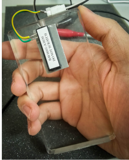
Fig. 7.2 Handheld mockup with a vibration actuator used in the user study.
