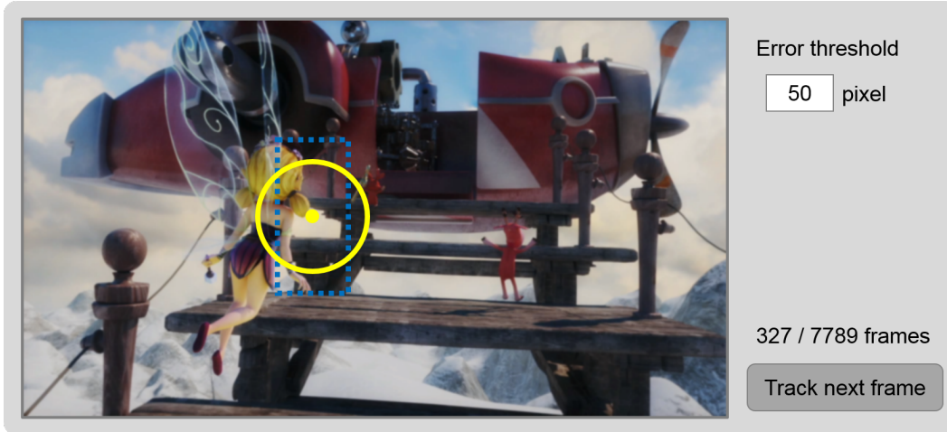
Fig. 6.1 Example user interface of interactive motion effects design. When the center of the object being tracked moves outside the yellow circle, the designer fixes its bounding box before clicking the ‘Track next frame’ button.
