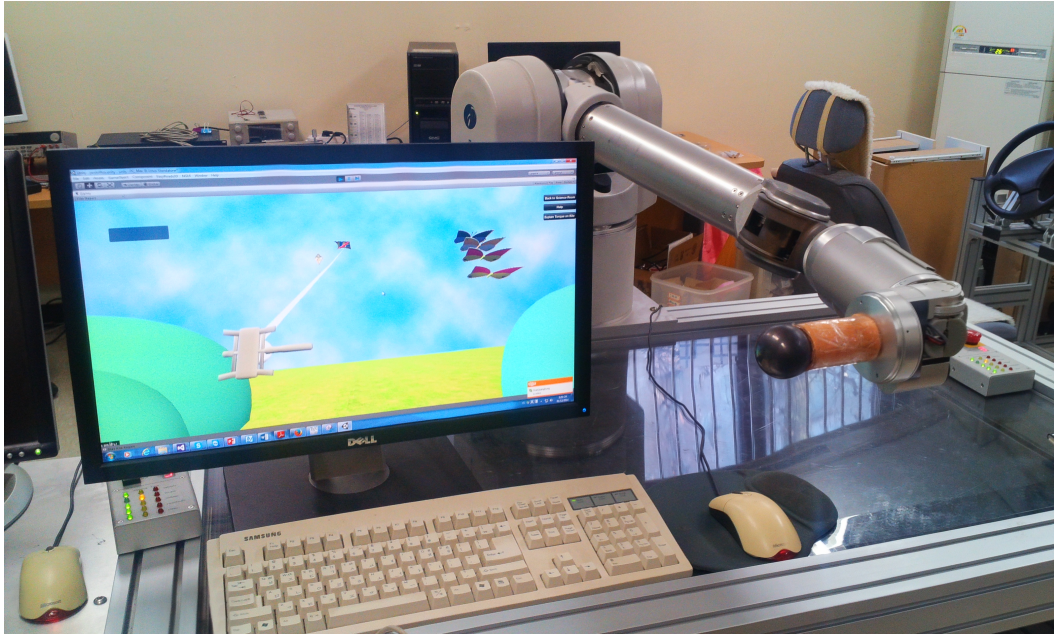
Figure 4.11: Haptic-enabled kite simulation using WAM arm device.
