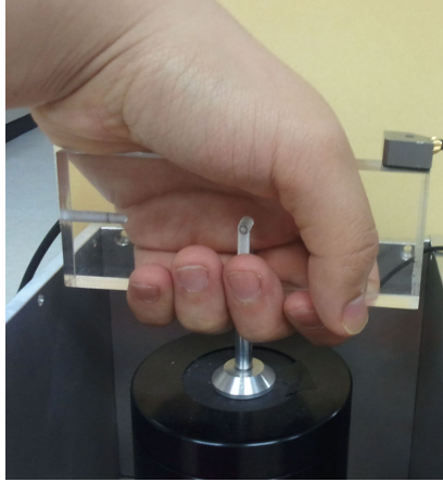
Figure 4.2: Mini-shaker with a mobile device mockup.
