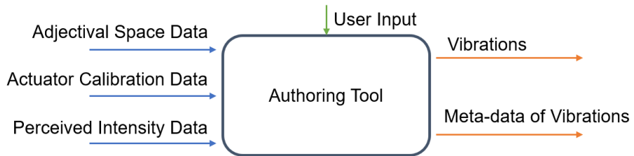
Figure 8.5: I/O scheme of the adjectival authoring tool.
