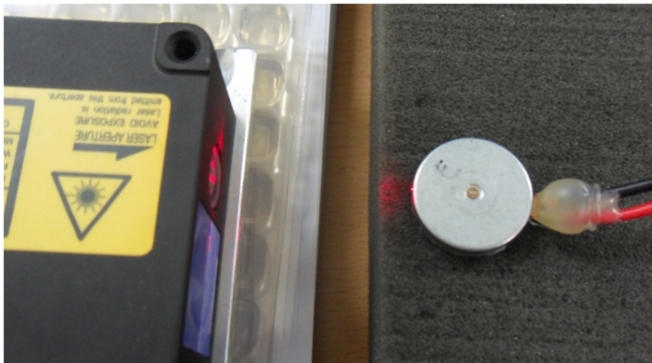
Figure 4.3 How the laser vibrometer is used to measure vibration
