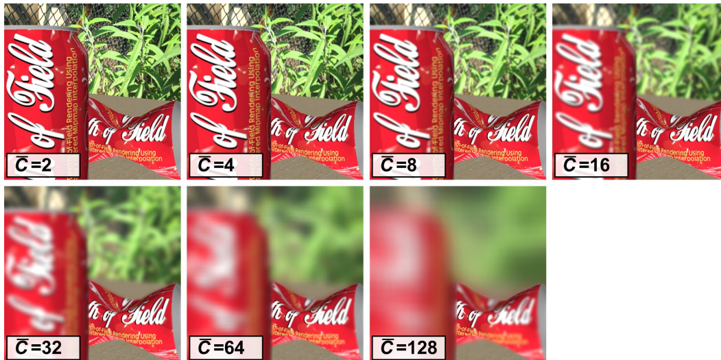
Fig. 4.13 The evolution of blurred appearance. When the mean CoC diameter ( \bar{C} ) is equal to or less than 16 pixels, the artifacts do not stand out.
