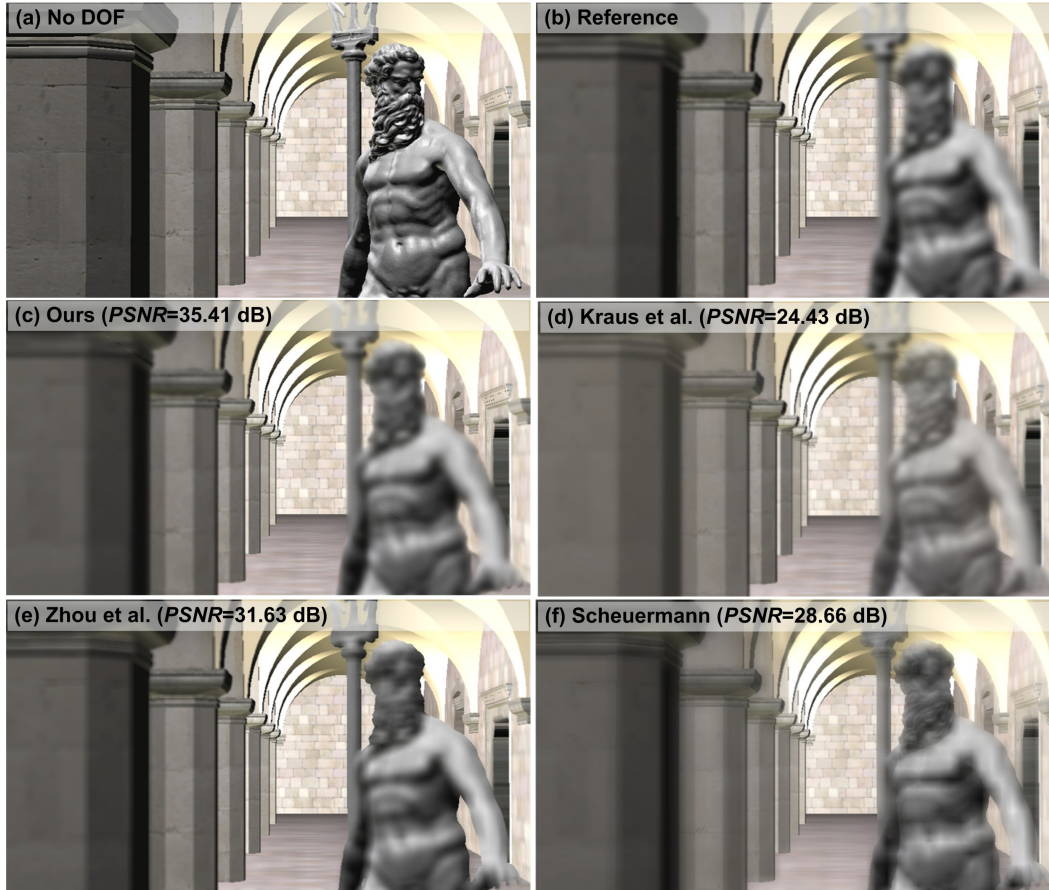
Fig. 4.12 A comparison of foreground-blurred images rendered by the same methods in Fig. 4.11. The farthest wall is focused.
