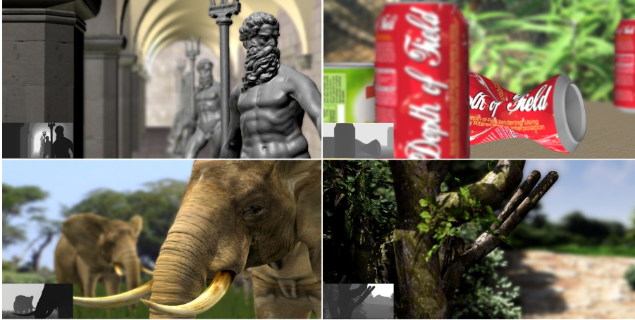
Fig. 4.1 Example images generated with our DOF rendering method and their depth maps (in the bottom-left corner of each image). The three scenes except the “Forest” scene (at the bottom right) were rendered in real time. The “Forest” scene was postprocessed in real time from an offline rendered image. Our method generates realistic DOF effects without any noticeable bilinear magnification artifacts, intensity leakage, and blurring discontinuity.
