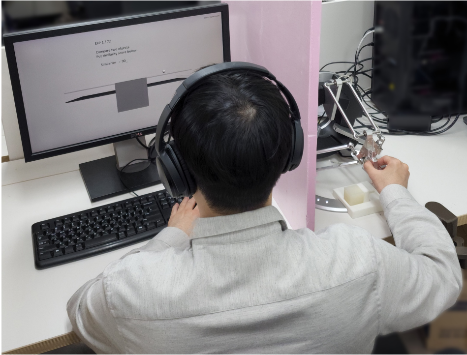
Figure 4.16: Setup of the perceptual experiment. A participant controls the force-feedback device while watching the monitor screen. The force-feedback device and deformable objects are visually blocked by the physical wall.
